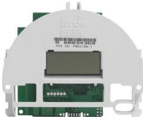
Figure 27: C1SR FCC Label Location
