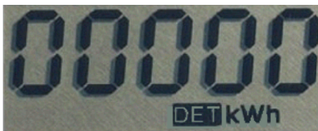
Figure 22: Delivered kWh with Detent Enabled
