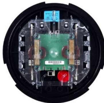
Figure 4: CENTRON 20 Amp Metrology
